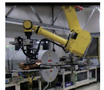
Automated inspection system utilizing an arm robot
