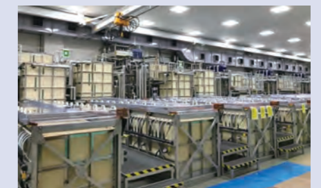
Production equipment used for semiconductor-grade sputtering targets such as electrolysis baths (Isohara Works)
