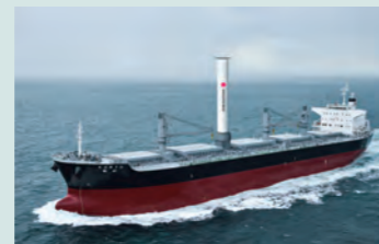
KORYU After the Installation of Rotor Sails
